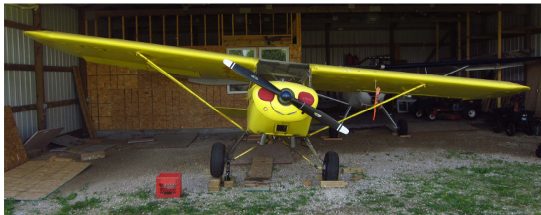
Figure 6: Calibrating unit by jacking the aircraft to each ball position
