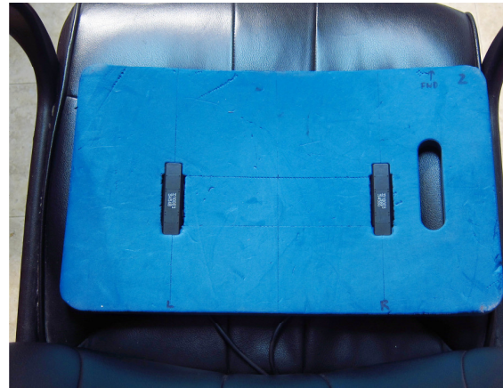
Figure 1: Seat cushion overlay (vinyl cover removed)
